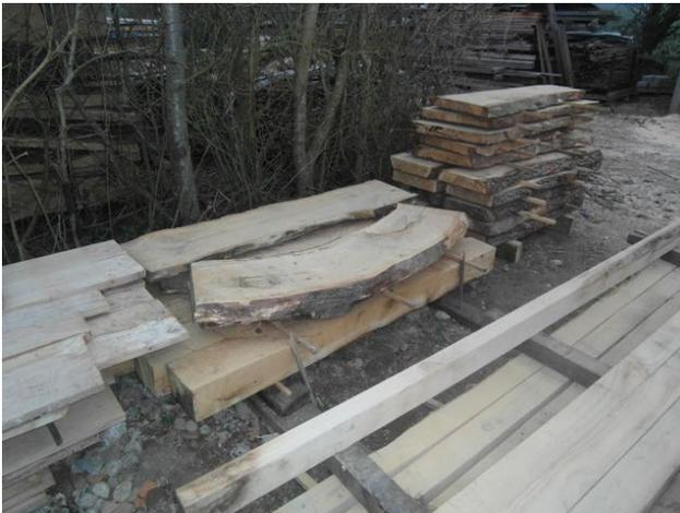
Pierre works with many local timbers: oak, chestnut, conifer, elm, poplar and sycamore. These are cut into lengths of 3.5 to 6m, for handling and storage, then moved to a mill where they are converted to the required size, before being moved for air drying in carefully stacked piles.
